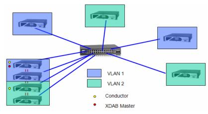
In this scenario, the network is divided into VLANs and an XDAB cluster is used. Two VLANs are shown; more are possible.
