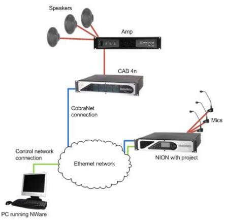
The control network and CobraNet network are both represented by a single *cloud*. You may choose to physically separate the wiring for the two networks, or logically separate the traffic using VLANs.
